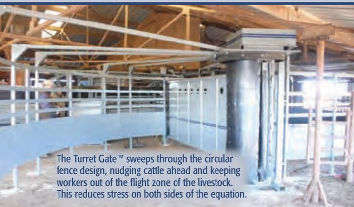
The Turret Gate™ sweeps through the circular fence design, nudging cattle ahead and keeping workers out of the flight zone of the livestock. This reduces stress on both sides of the equation.
